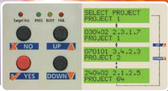
The FS2009USB programmer being used in standalone mode
