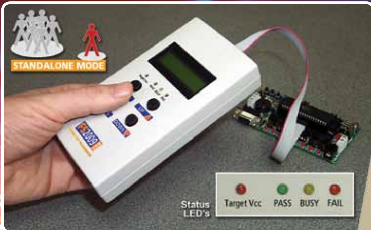
The FS2009USB programmer being used in standalone mode
