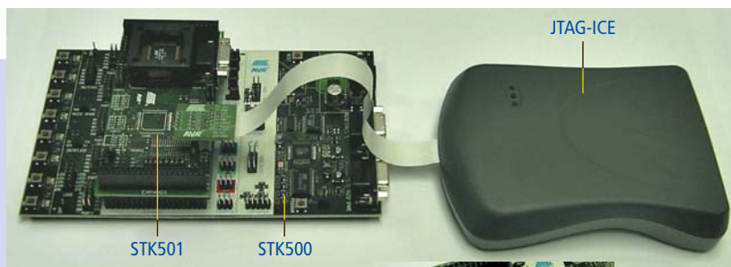
A typical ATmega128 Development System: The STK501 is plugged into the STK500 board and the JTAG-ICE connects to the JTAG Port on the STK501
