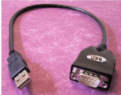
One end of the '**USB to Serial Cable**' plugs into a spare USB port on the host PC. The other end connects to the 'Serial Port' on the Equinox Programmer. This application note describes how to connect the Equinox '**USB to Serial Cable**' and how to install the USB Driver software onto your PC to support this cable.
