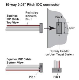
The **CAB-ARM-10W-150** is an In-System Programming (ISP) ribbon cable designed to connect from any ISP programmer which features a 10-way 0.05" pitch connector to a 10-way 0.05" pitch connector on a suitable ARM microcontroller Target System. The cable features 150 mm of flat ribbon cable with a 10-way 0.05" (1.27mm) pitch female connector on each end.
