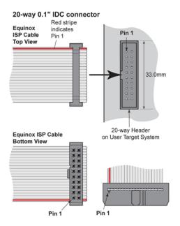
The **CAB-ARM-20W** cable is a **20-way** In-System Programming (ISP) ribbon cable designed to connect from any ISP programmer which features a 20-way IDC connector to a 20-way 0.1" pitch IDC connector on a suitable ARM microcontroller Target System. The cable features 200mm of flat ribbon cable with a 20-way 0.1" pitch female IDC connector on each end. The IDC connectors are fitted with 'cable grips' and are bump polarised to prevent the connector being plugged in the wrong way around.
