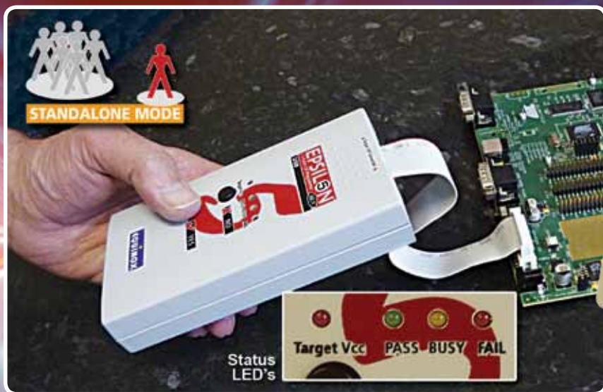
The EPSILON5-MK4(ARM) programmer being used in Standalone Mode
