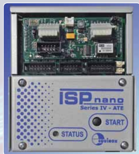
IOMOD14 module shown connected to an ISPnano Series 4 programmer. The programmer is NOT supplied with the IOMOD14 kit
