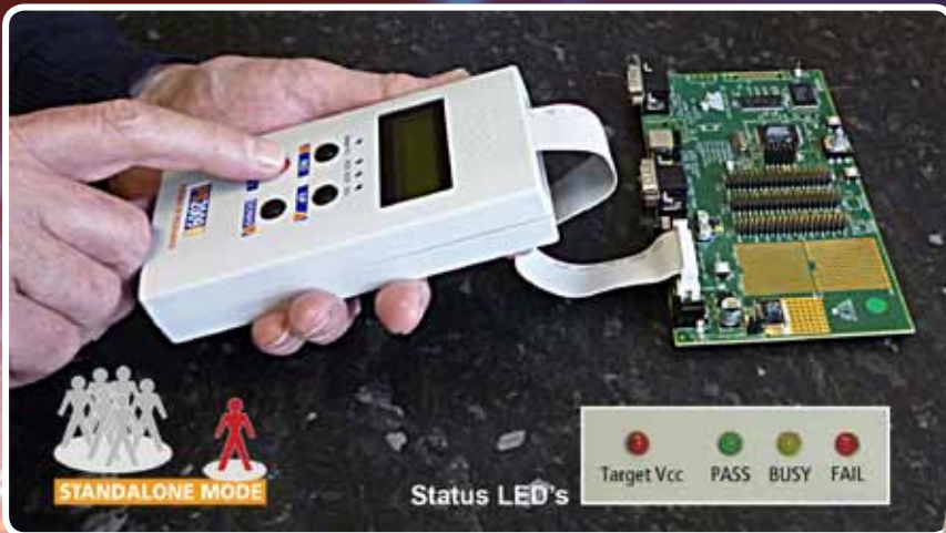
The FS2009USB (ARM) programmer being used in Standalone Mode
