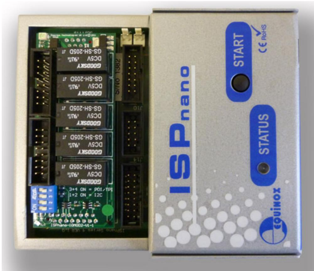
The programmer supports automated relay switching of all Target System programming and power signal lines between external test equipment e.g. an external ATE / ICT system and the programmer. This allows the programmer to be completely out-of-circuit during normal ATE testing operation.
