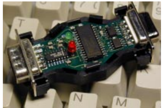
Top side (in enclosure) with Philips SJA1000.
