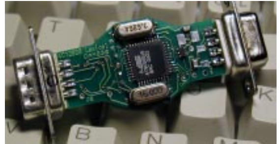
Bottom side with Atmel 8515 AVR.
