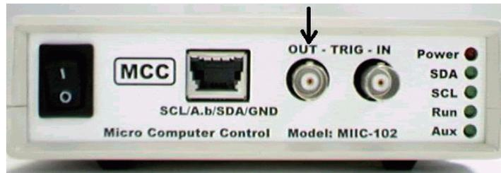
The Trigger Out port is optionally used to synchronize external equipment with I<sup>2</sup>C Bus events or data match pattern. This port is located on the front of the pod, and uses a BNC type connector. Output lines are provided for signal and ground.
