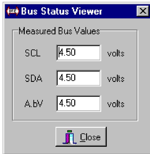
Use the Bus Status Viewer dialog box to view the current voltage levels on the I<sup>2</sup>C Bus Clock, Data, and A.bV lines. This viewer is useful in determining if the Clock or Data lines are stuck low.
