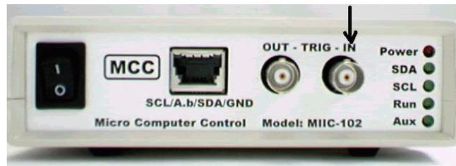
The Trigger In port is optionally used to synchronize I<sup>2</sup>C Bus data collection with an external event. This port is located on the front of the pod, and uses a BNC type connector. Input lines are provided for signal and ground.
