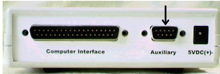
The Auxiliary port is used to connect the I<sup>2</sup>C Bus Monitor pod to external equipment. This port is located on the rear of the pod, and uses a DB-9M type connector. Auxiliary lines include:
