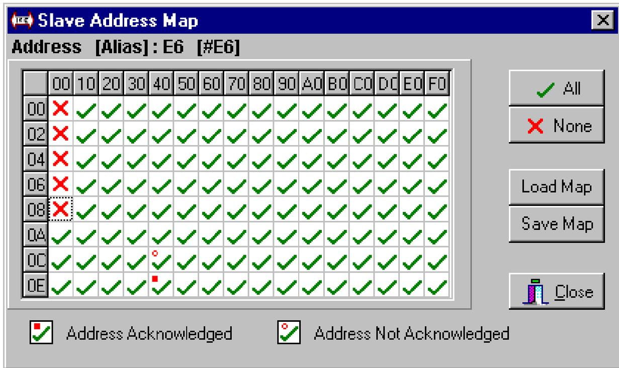
Use the Slave Address Map dialog box to select I<sup>2</sup>C messages to display by Slave Address, and to globally monitor all address activity.
