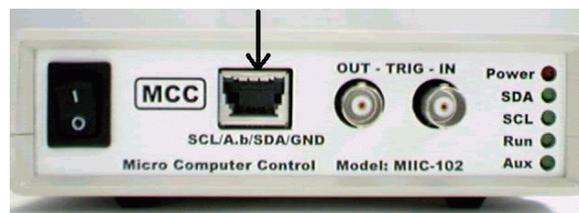
The I<sup>2</sup>C Bus port is used to connect the pod to the I<sup>2</sup>C Bus under test. This port is located on the front of the pod, and uses a Molex ACCESS.bus type connector. Input lines are provided for I<sup>2</sup>C Clock, Data, and Ground, and System Under Test Vcc voltage measurement.
